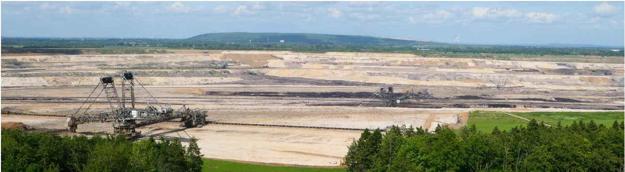
Figure 7 View of an active lignite open pit mine (Inden, North Rhine-Westphalia). In the distance a large artificial hill (16 km 2 , 200 m tall), the so-called Sophienhöhe, is created by the disposal of 1,100 Mt spoil from the Hambach lignite mine. The mine opened in 1978, and the first tree was planted the same year. Since then, much of the spoil hill has been forested with 10 million trees, and the entire hill has become a recreational area with a > 120 km-long network of hiking trails. Such recultivation gained international recognition and was awarded in 2020 as part of the United Nations Decade on Biological Diversity
