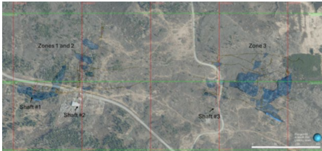
Figure 4 Surface openings mine hazards location (blue zones are the stopes)
