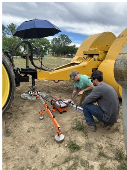
Figure 6 Variable energy dynamic penetrometer – PANDA
