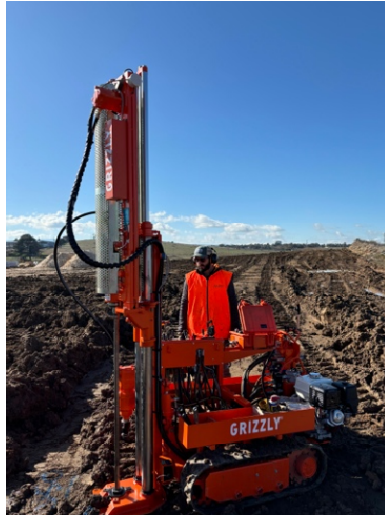
Figure 5 Dynamic probing super heavy – GRIZZLY rig
