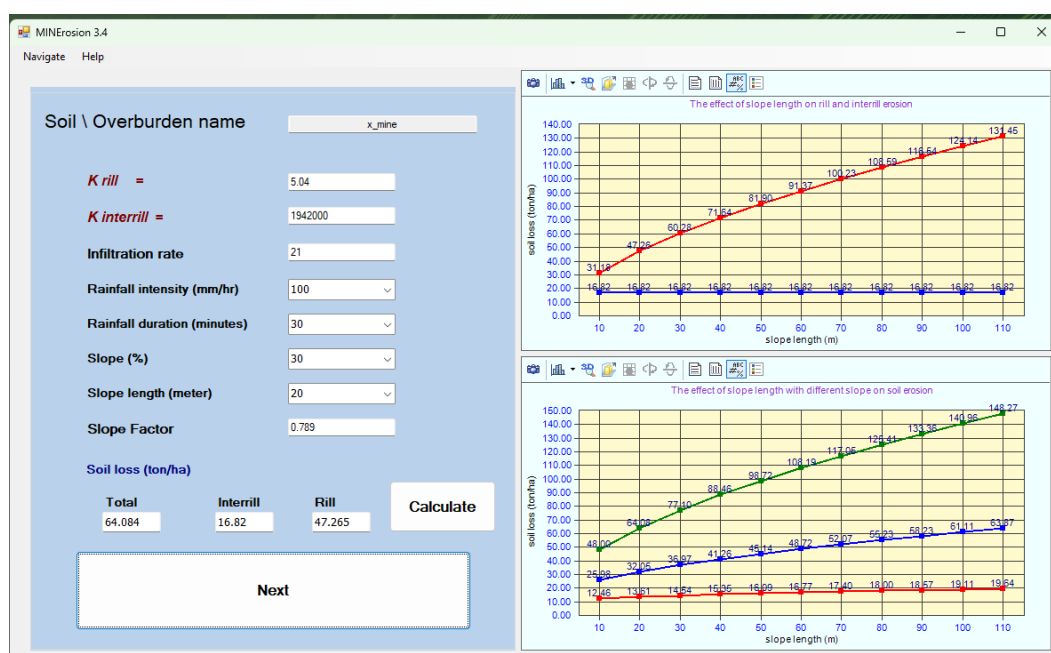
Figure 1 MINerosion 3.4: estimation of rill and interrill soil loss (t/ha), showing the effects of slope length and gradient using the model's graphical interface
