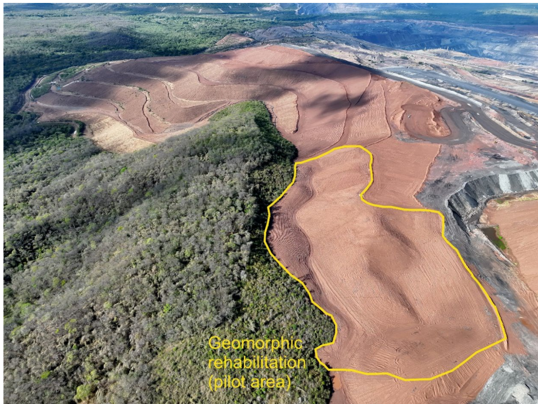
Figure 3 Aerial view of the geomorphic rehabilitation pilot area of the Annex waste rock dump, showing the traditional, benched landform design in the background. Image taken on 25 December 2025
