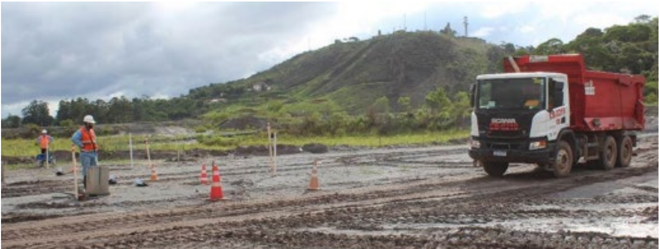
Figure 6 Damping tests of dump truck operations to characterise vibration decay in tailings (Ramos et al, 2023)
