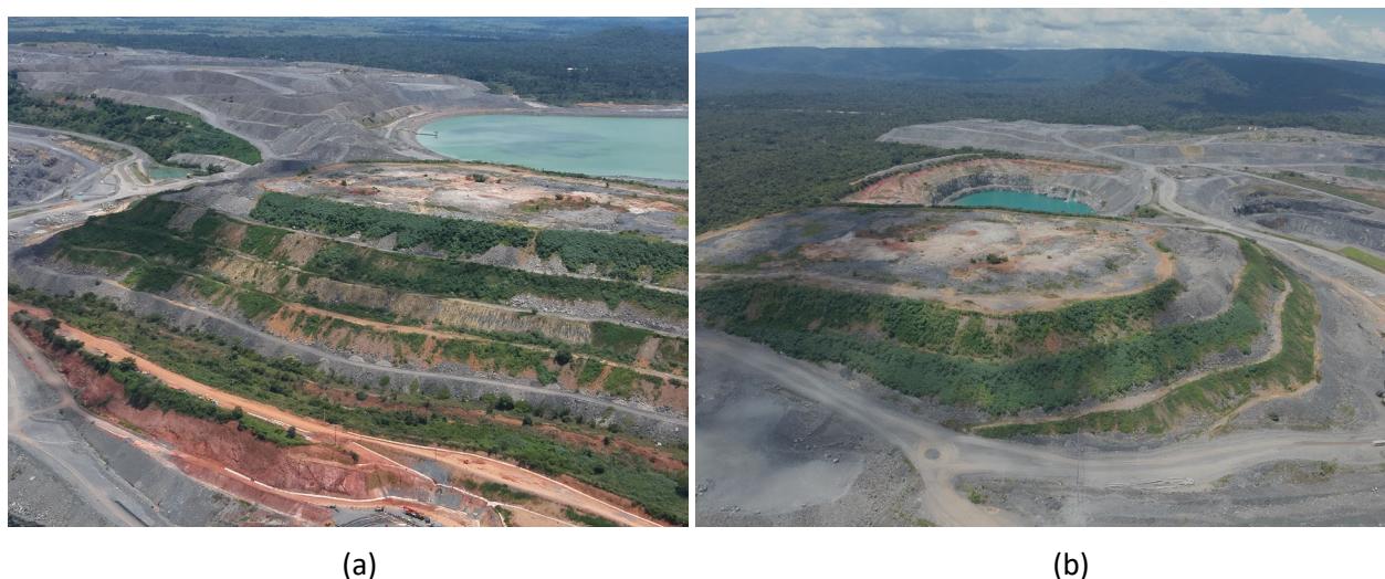
Figure 11 Revegetation progress after progressive closure interventions; (a) Southwest waste rock pile; (b) North waste rock pile
