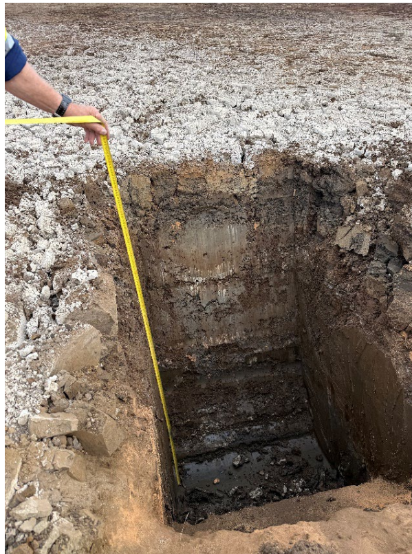
Figure 3 Test pit excavated in Cell 1 tailings
