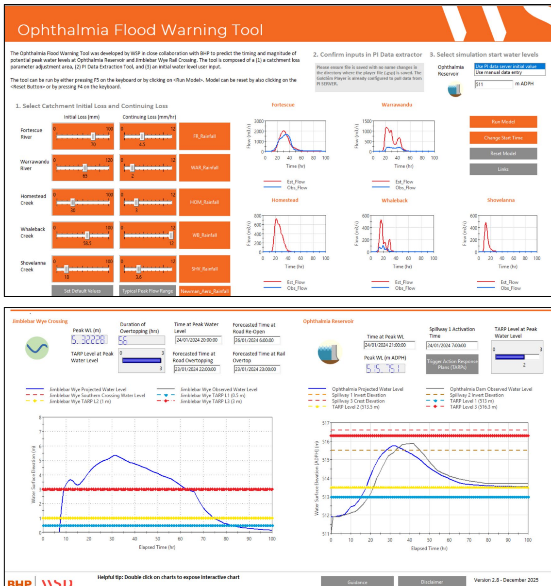
Figure 9 Model user interface and decision support outputs. TARP = trigger action response plan, WL = water level
