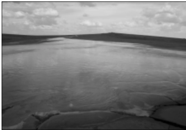
Figure 8: Sheet flow characteristics of paste, after initial channel flow.
