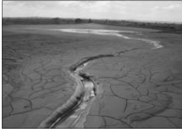
Figure 7: Paste is directed down a water-formed channel to the desired area of deposition.
