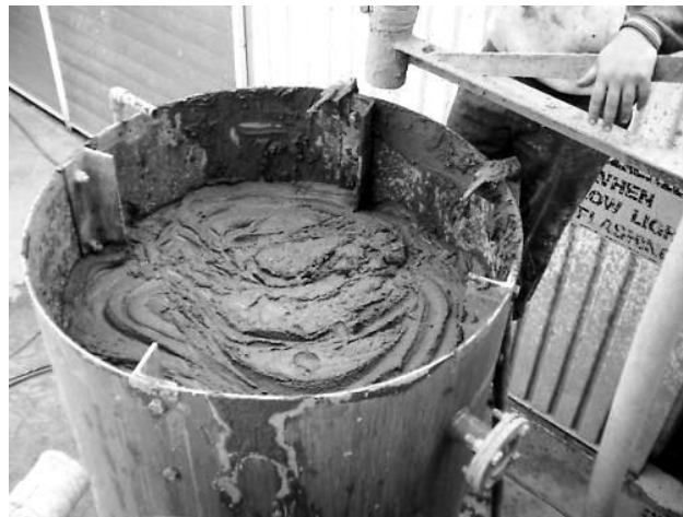
Figure 1 Non-Newtonian thickened tailings ( \tau_y = 70 Pa, K_b = 0.060 Pa.s)
