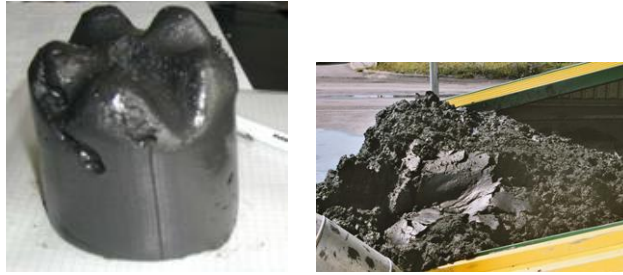
Figure 8 Coal paste from Siersza where a feeding auger is required
