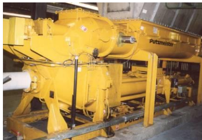
Figure 9 KOS pump with feeding auger at the coal power plant Siersza
