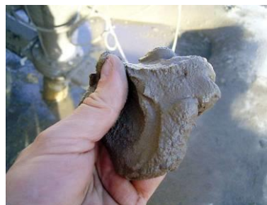
Figure 7 Fine grained backfill paste of Plutonic Gold Mine
