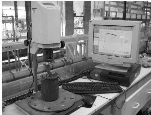
Figure 2 Rotary viscometer with vane attachment
