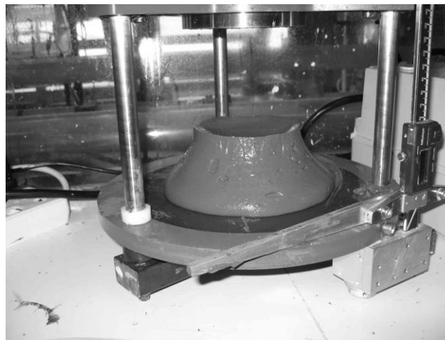
Figure 8 Typical slumped cone formed by kaolinite tailing
