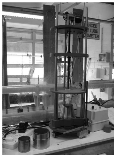
Figure 1 The new slump meter with lift speed control
