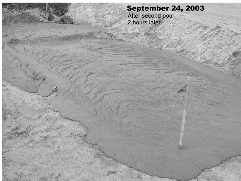
Figure 4 MFT drying field trial — initial deposit
