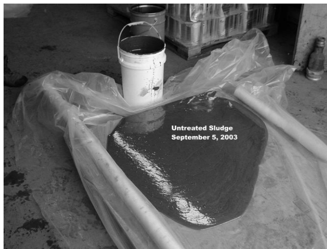
Figure 2 Untreated MFT on 4% slope
