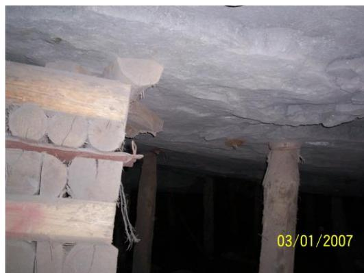
**Figure 4** Conditions in Panel 6N. Significantly less closure and ride was observed in this panel as it was being mined in overstoped ground
