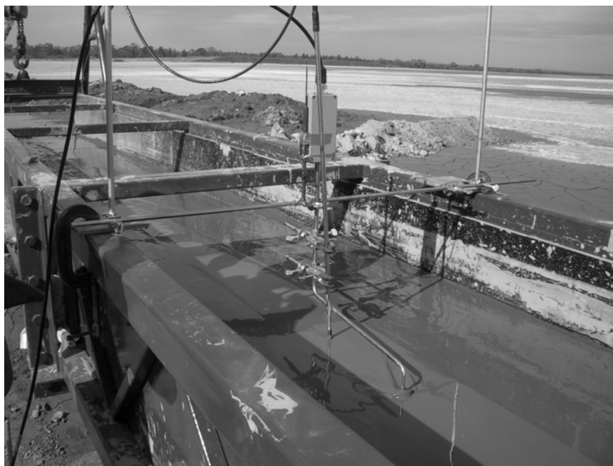
Figure 8 Velocity and density probes being immersed into the tailings channel in the flume
