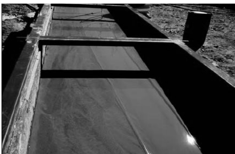
Figure 7 A self-formed channel in a bed of freshly deposited tailings
