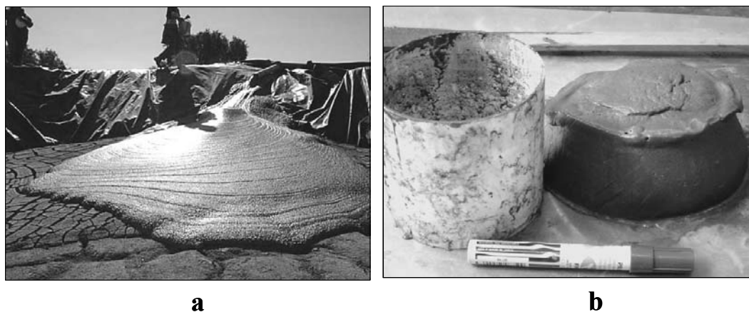
Figure 1 a) Surface disposal of industrial mineral paste, Vietti and Dunn (2002); b) Slump laboratory cylinder, Hernández et al. (2005)
